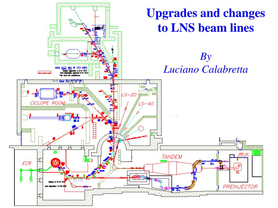
To deliver the new high power beam to the existing beam lines we need a 90° bending magnet and at least further 4 quads and dedicated diagnostic.
