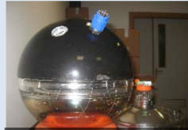
The OM: 10" Hamamatsu R7081, Front End Module, Time Calibration, LED beacons
