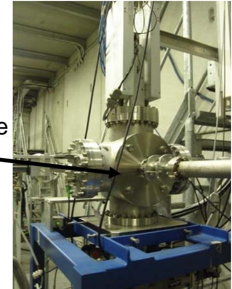
**Micro channel plate** in front of a X-Y electron **collecting anode**: current from 10fA to 1 nA: radioactive beam
