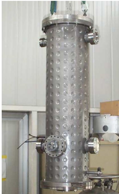
Fig. 4 . Photo of existing 80 MHz PIAVE buncher
