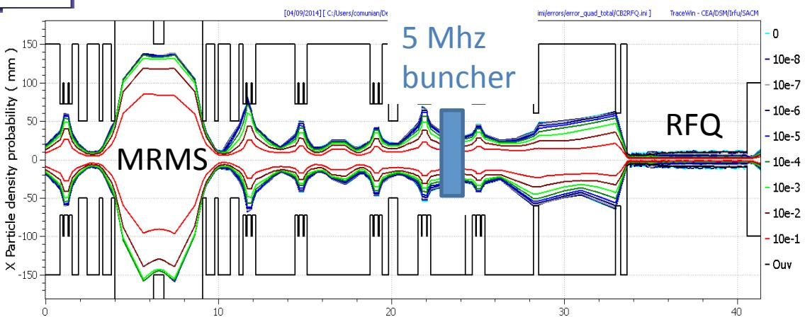
Total amount of space occupied by the beam due to quad errors
