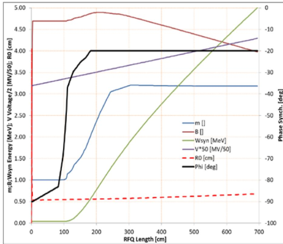
Figure 1: The main RFQ parameters vs. length.
