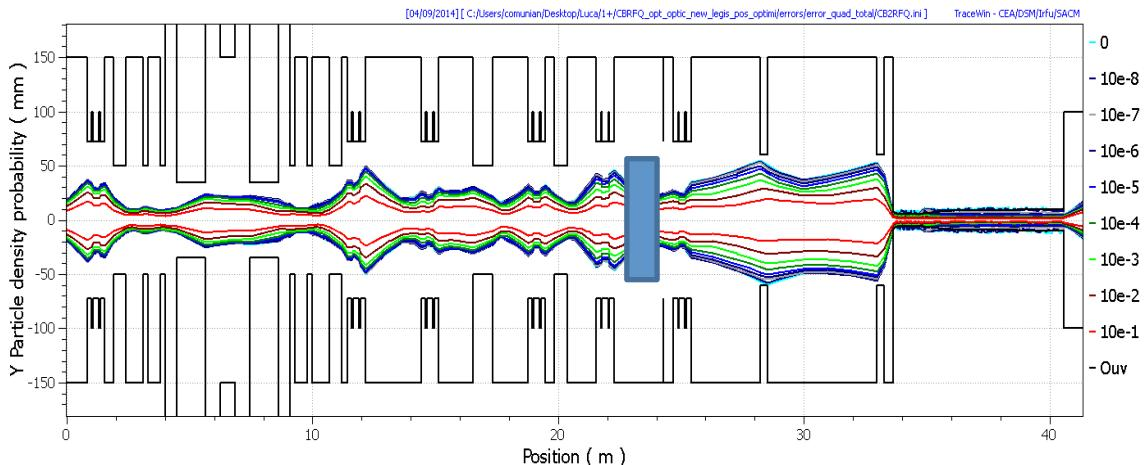
Without buncher: total losses 93-94 % after the RFQ, output longitudinal emittance 0.067  $\pi$ mmmmrad.
