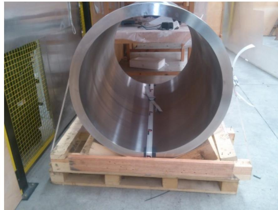
Bolted electrodes, copper plated 304L tank,
