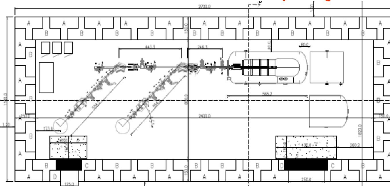
Preliminary project of installation and shielding: 1.5 m concrete for lateral walls and 1.3 m concrete for roof.
