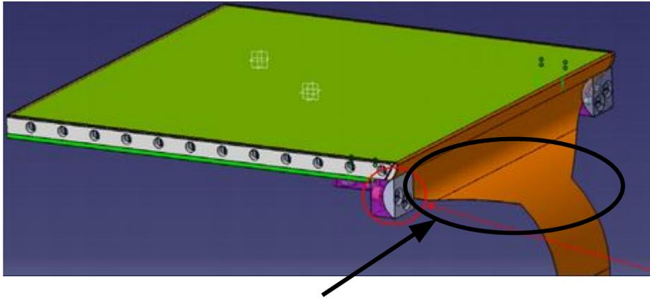
We avoid use of non-radiopure connector here. Just extension of kapton-copper foil with readout lines.
