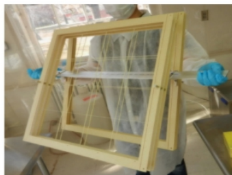
Frames on a custom holder for cleaning in Ultrasonic bath
