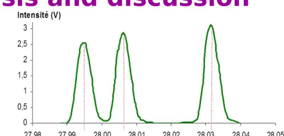
Example of high resolution mass spectrum. 12 C 16 O, 14 N and 12 C 14 H 2 can be separated
