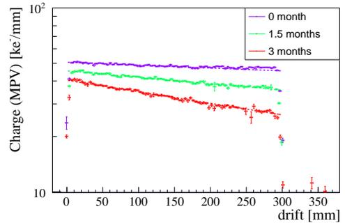
**Figure 6.** Charge as a function of the drift distance, for three runs, 6 weeks apart, normalised to the reference run 2008.
