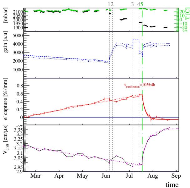
**Figure 7.** Time evolution of the gain, of the attenuation and of the drift velocity. We can see several variations of the gain due to the pressure loss when gas samples were extracted. For the first five months during which the TPC was sealed we see a regular degradation of all three parameters. On July 20 (line 5), the CAPS was turned on.
