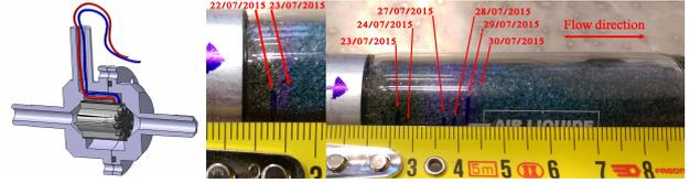
**Figure 2.** (Left) Sectional view of the circulator (CEA patent BD15730SG). (Right) Picture of the Oxisorb cartridge after 10 days of continuous use.
