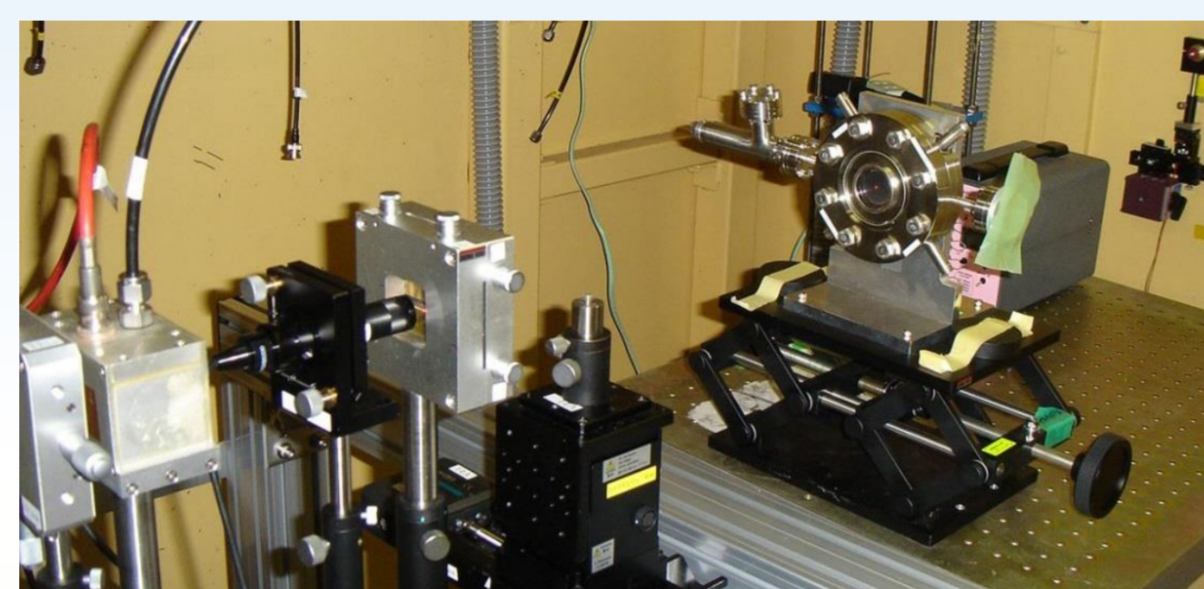
The energies of the incident X-ray beams were fixed at 6 keV by a Si double-crystal monochromator. The incident X-rays were defined by a collimator of 0.1 mm diameter.
