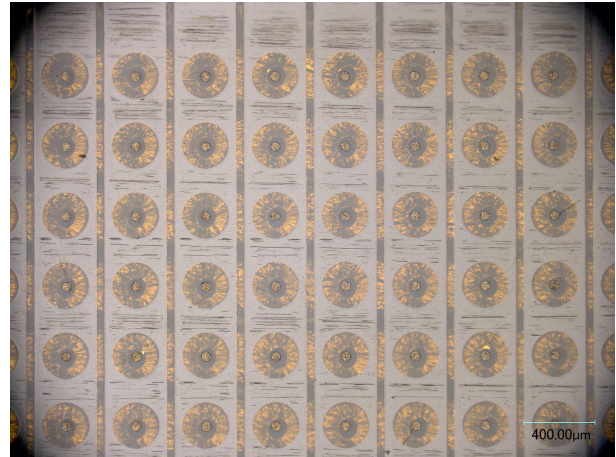
Figure 5. Microscopic image of a new prototype. The readout pitch is 400 µm. Pixels are well aligned, and carbon sputtered cathodes are properly formed in the entire detection area.
