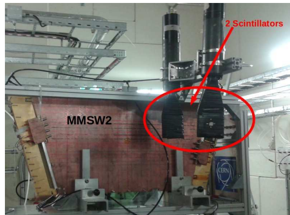
Figure 4. MMSW2 detector plus the two scintillators used for the trigger signal.
