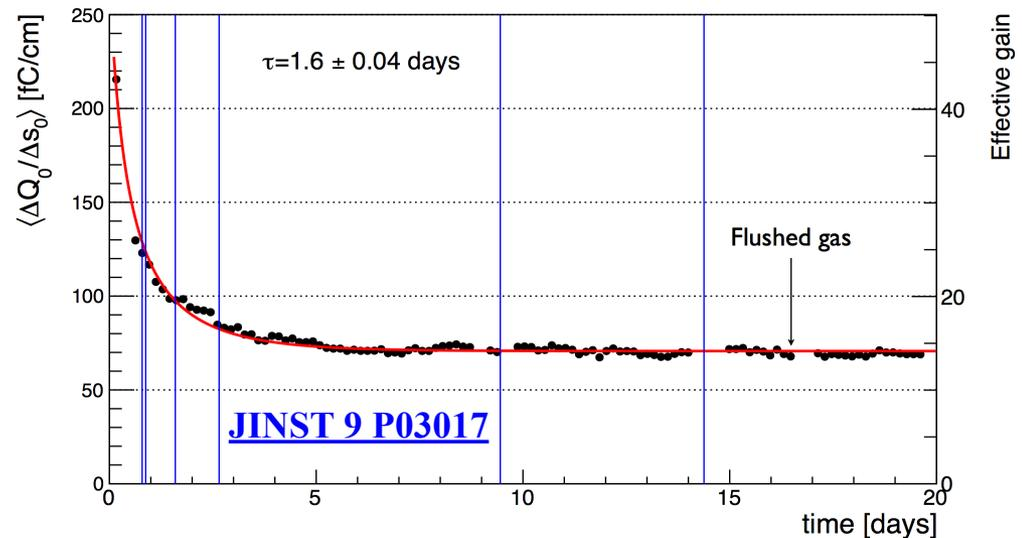
Discharge voltage improves with charging-up in the 40x76 cm<sup>2</sup> (250 L) LEM test
