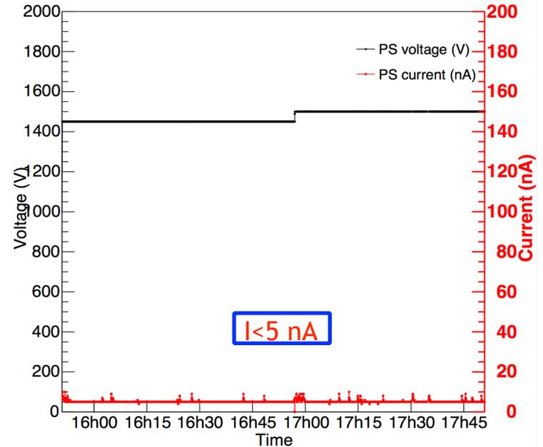
Discharge rate in Ar(90%)+CO<sub>2</sub>(10%)
