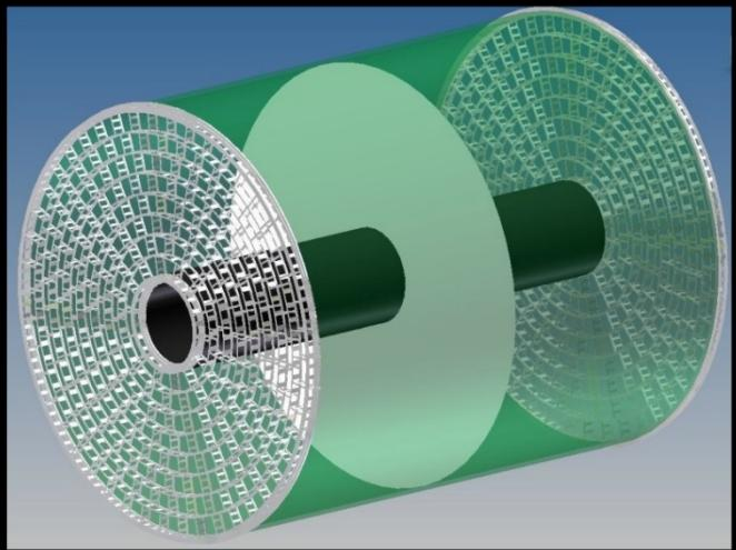
Primary ions create distortions in the electric field →  $O(10\mu\text{m})$  track distortions
