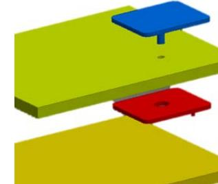
Pad anode with capacitive coupling pad readout
