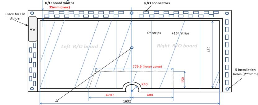
For tracking in technical run in beg 2016 plan to have 4+1 detectors  $66 \times 41 \text{ cm}^2$  and detector  $163 \times 45 \text{ cm}^2$
