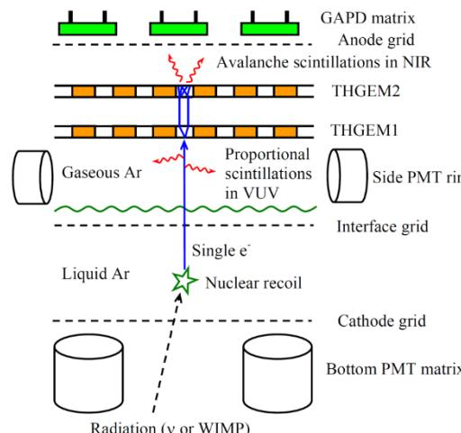
THGEM/GAPD-matrix multiplier with PMT readout of proportional EL of the ionization (S2) signal
