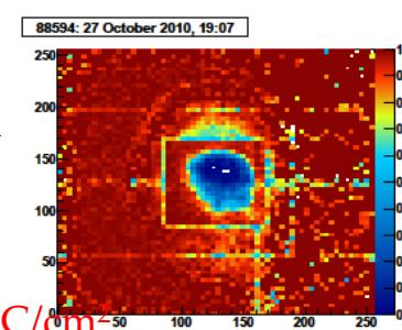
Tracked down to Si deposits on GEM; culprit were **gas leaks** that allowed Si from an **outside sealant** to migrate into chamber →
