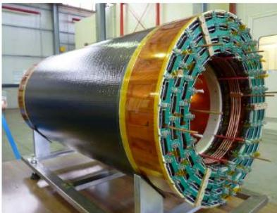
The final assembly of the KLOE-2 Inner Tracker, with the insertion of all the triple-CGEMs one into the other took place in March 2013
