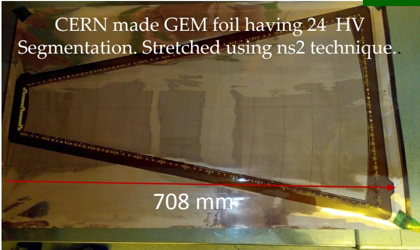
CERN made GEM foil having 24 HV Segmentation. Stretched using ns2 technique.
