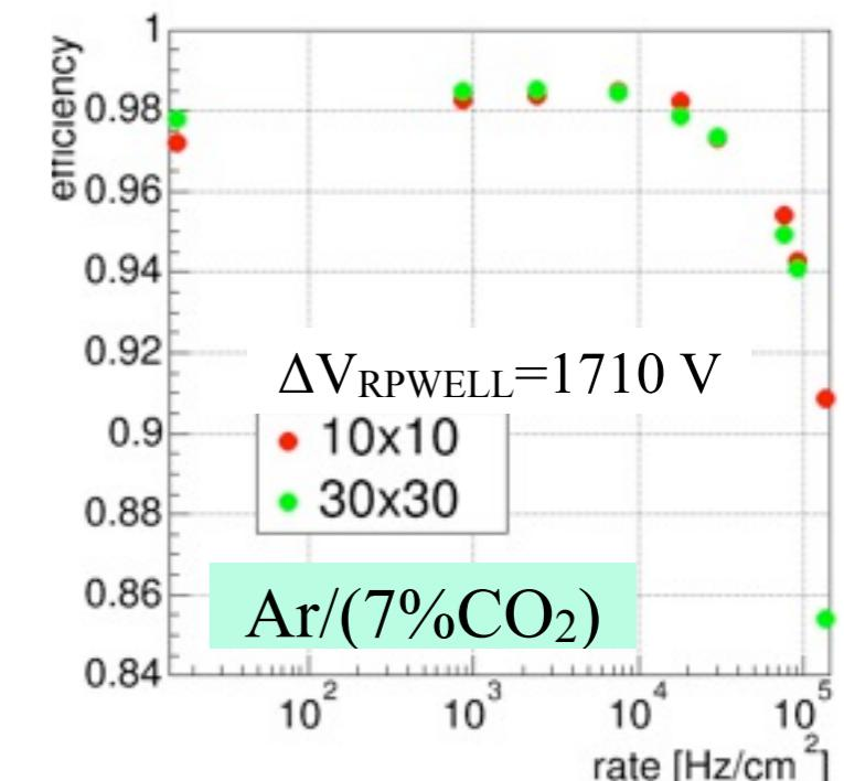
$10 \times 10 \text{ cm}^2$  - Discharge-free operation also at high rate  $\pi$ -beam
