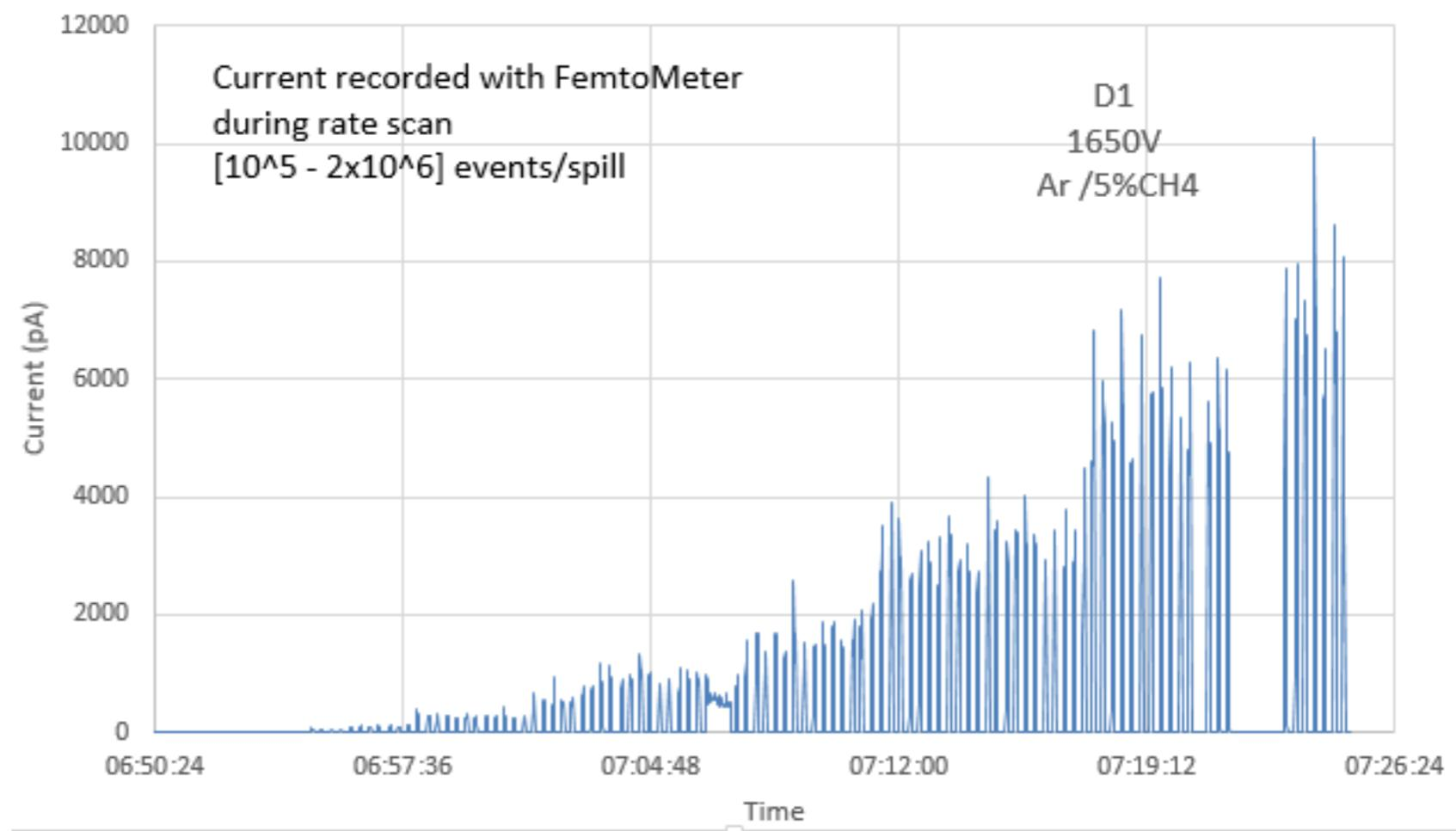
10×10 cm<sup>2</sup> - Discharge-free operation also at high rate  $\pi$ -beam
