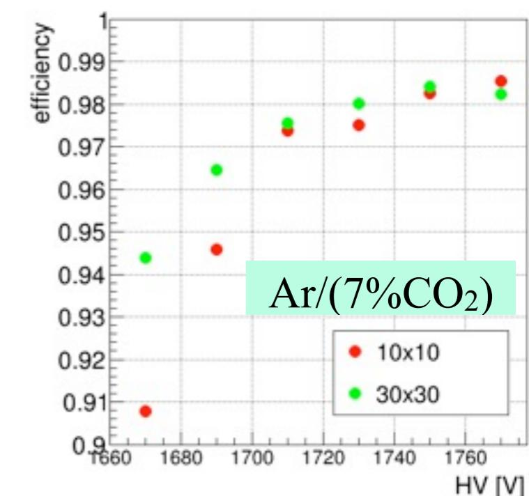
$10 \times 10 \text{ cm}^2$  - Discharge-free operation also at high rate  $\pi$ -beam
