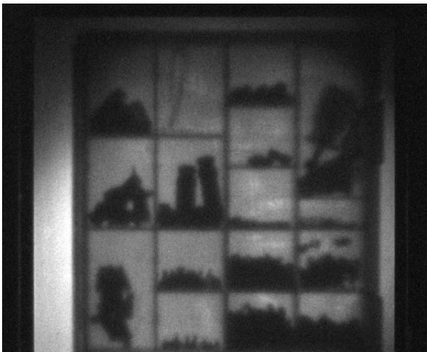
Figure 9. X-ray transmission image of a tool box obtained by large size scintillating G-GEM detector with an x-ray tube voltage of 25 kV, current 50 \mu\text{A} . Effective area of the x-ray image is 280 \times 280 \text{ mm}^2 . The image was taken with an exposure time of 5 seconds (gas gain: 3,000).
