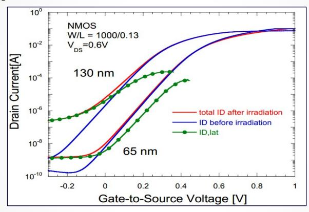
A larger amount of lateral leakage takes place in 130 nm devices
