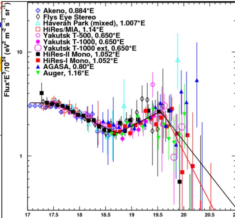
● Fluxes are extremely low and the challenge is to build an instrument able to detect a few particle per km<sup>2</sup> per century.
