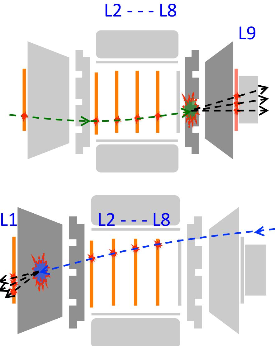
First, we use the seven inner tracker layers, L2-L8, to define beams of nuclei: He, Li, Be, B, ...
