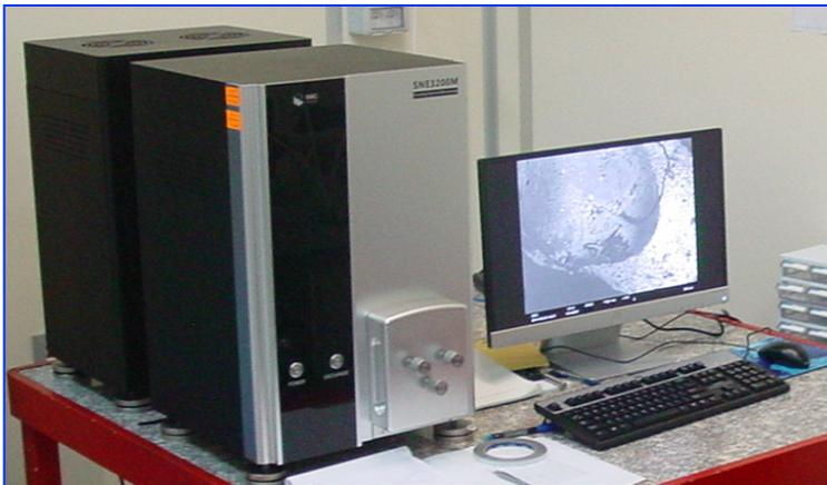
*Table-top Scanning Electron Microscope (mini-SEM)*
