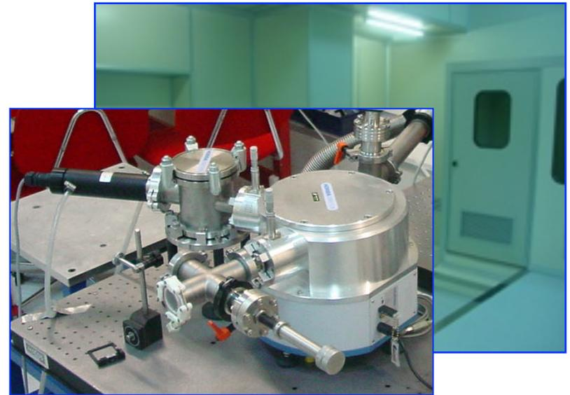
Instrumentation has been upgraded with a new *VUV monochromator* (UVXL200 by Jobin Yvon) operating in the 120-250 nm spectral range. The other monochromator operates in the range 200-650 nm.
