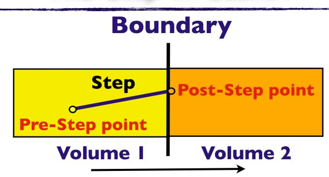
The G4Step contains the information about the Pre-Step point and the Post-Step point and the "variation " of a physical quantity in the step (i.e the energy loss on the step). To access these information or objects instance it is possible to use manu Get method of the G4Step class:
