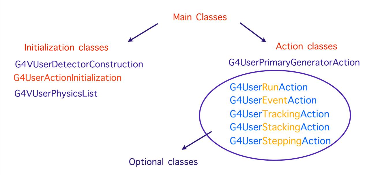
$\checkmark$  Five (or more) concrete base classes can be implemented by the user, adopering the virtual member functions to obtain the control of the simulation at various stages
