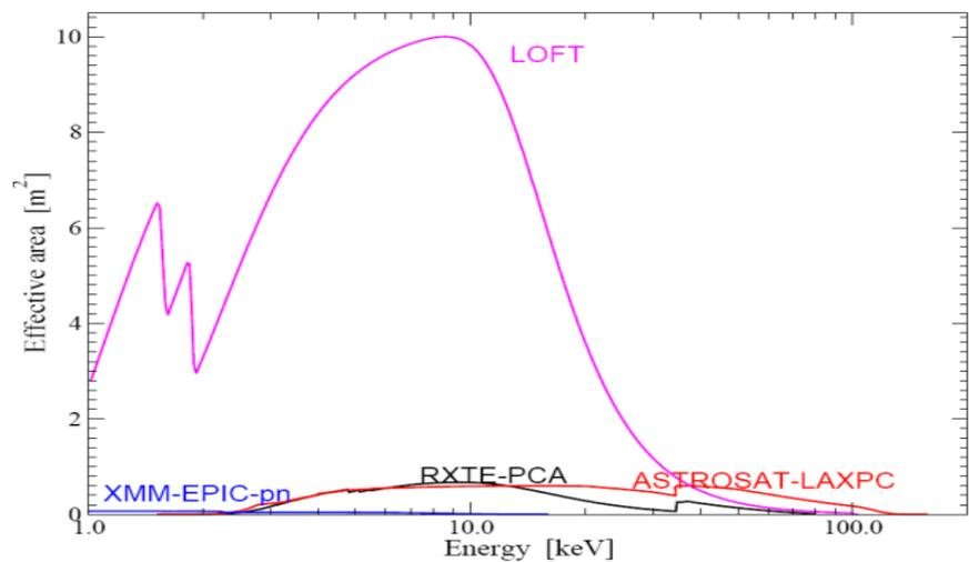
Far the best measurements of timing were performed by XTE PCA, that served for 15 years til 2010. LOFT Large Area Deector is 20 times PCA.
