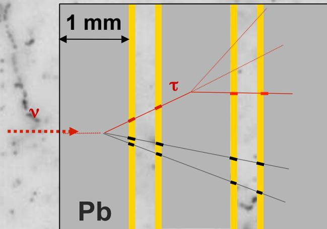
The OPERA target consists of 150'000 ECC bricks.
