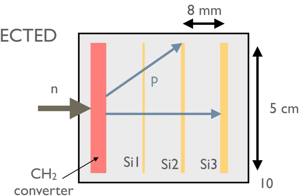
G. Ban et al., "A telescope for monitoring fast neutron sources", NIM A 577 (2007) 696-701
