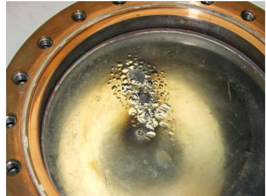
SARAF phase-I Tungsten beam dump after irradiation by  $\sim 10 \text{ mA}^*\text{hr}$  protons at 2-3 MeV
