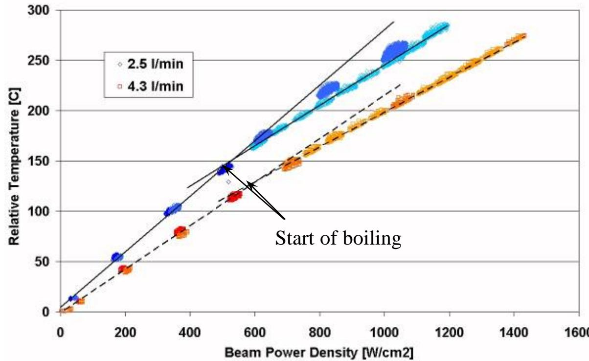
Measured wall temperature above coolant temperature as function of heating power flux for two flow rate. Distinctive change in heat transfer capability can be noticed at power flux of about 600 W/cm<sup>2</sup>. Stable operation has been achieved for heating power of up to 1400 W/cm<sup>2</sup>
