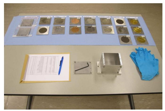
→ B, Mn, Co, Cu, Nb, Rh, W, Au samples with different thicknesses Selection of samples by DG-ENER, IAEA and DOE representatives
