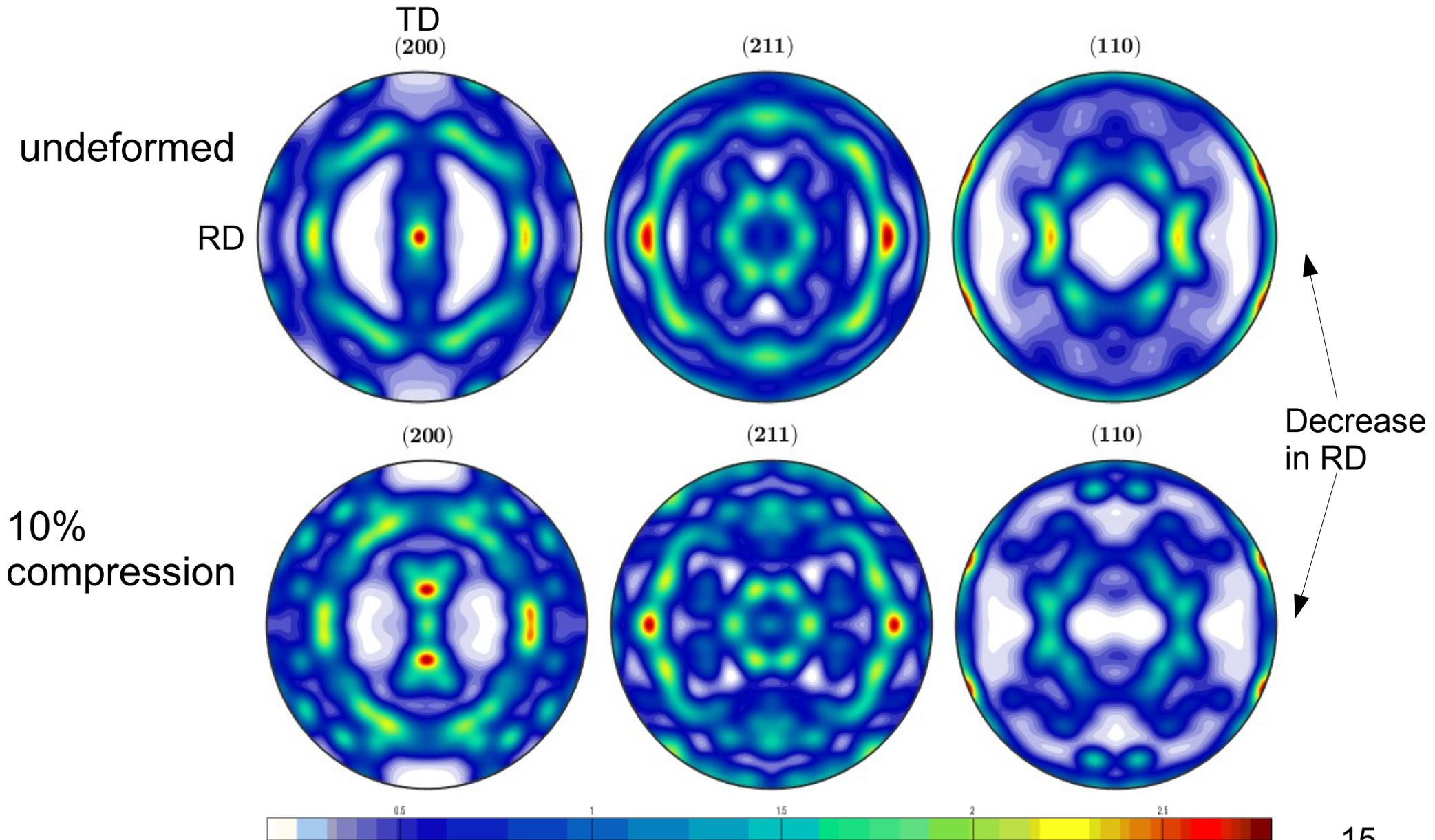
They are changed due to compressive deformation
