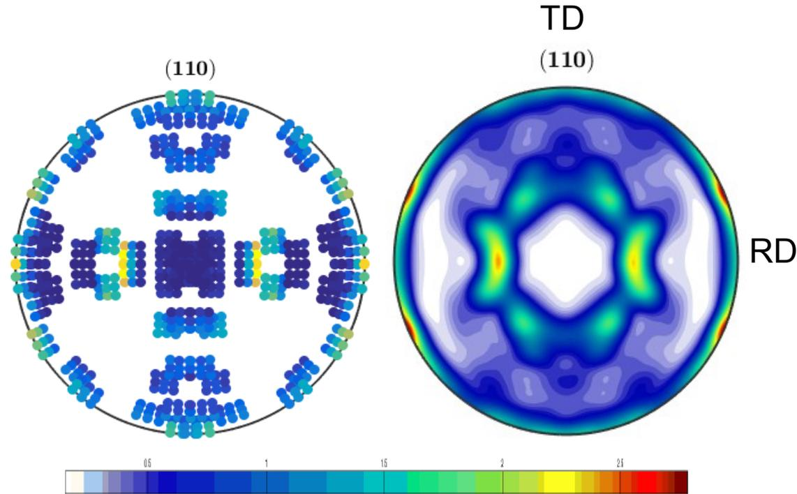
21 diffraction measurements covered a quarter of pole figure. It is complemented with ODF (mtext-4.0.12)
