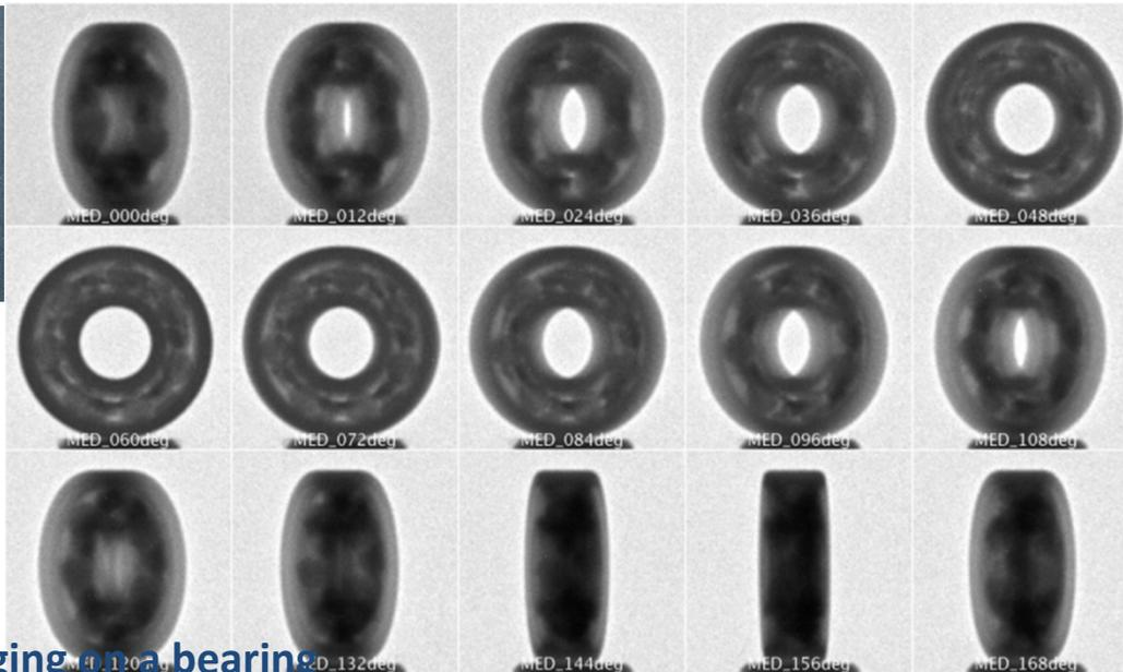
**Test of CT imaging on a bearing**
