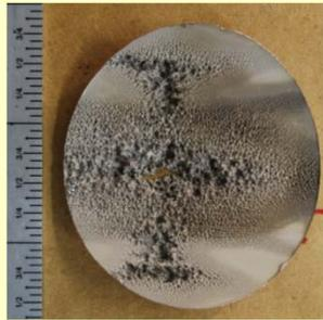
**Pitting Damage on a SNS target**
