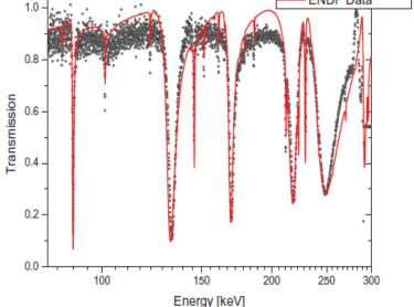
Inelastic neutron scattering cross-section measurements on actinides - GRAPHEME
