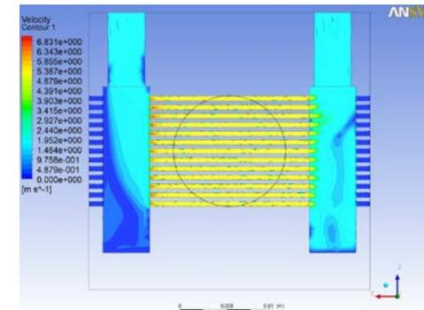
$\mu\text{-channel fluid velocity} = 5\text{ m/s}$
