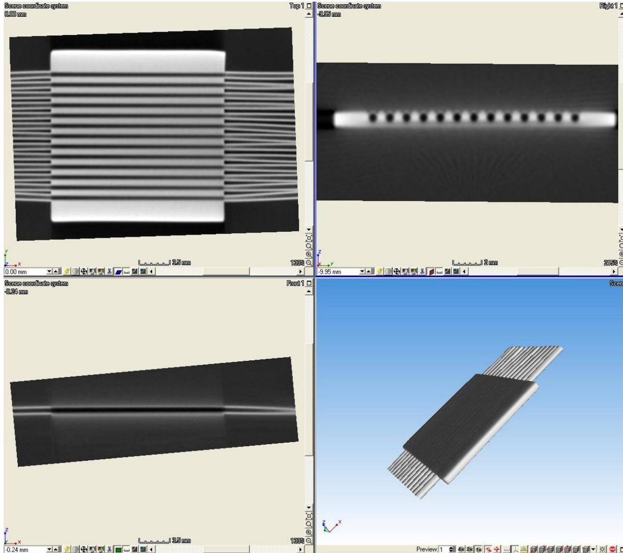
Certified an almost perfect contact (no defect at the 1  $\mu\text{m}$  level precision)
