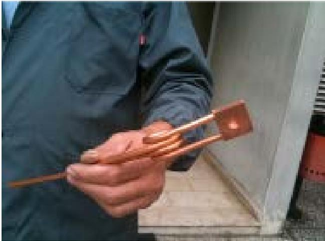
Micro-channels produced with electro-erosion drilling machine.
