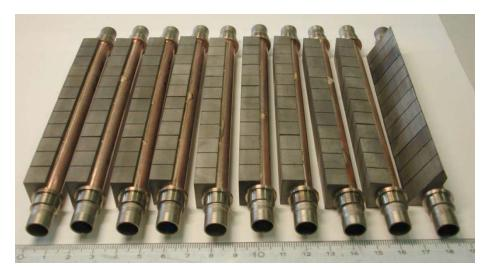
1. Be tile brazed cooling pipes
