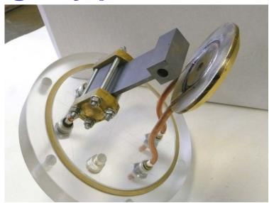
Be element equipped with collimator to simulate the proper proton hitting angle on target surface with same power density
