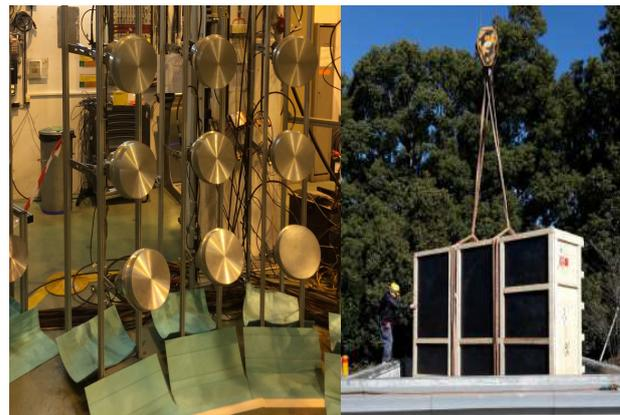
**Fig. 15.** Left: Neutron detectors, to be used at FAIR, during a recent experiment on <sup>11</sup>Li at ISOLDE. Photo: B. Jonson. Right: Neutron detector planes for the future NeuLAND at FAIR shipped to RIKEN for measurements of <sup>26–28</sup>O.
