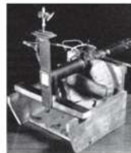
Figure 1.5 Parabola mass spectrograph constructed by J.J. Thomson (1910) with a discharge tube as ion source, a superimposed electrical field and a magnetic field oriented parallel to it for ion separation, and a photoplate for ion detection. (H. Kienitz (ed.), Massenspektrometrie (1968), Verlag Chemie, Weinheim. Reproduced by permission of Wiley-VCH.)
