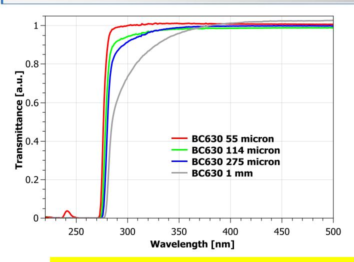
Transmittance curves normalized by the single- quartz support spectrum
