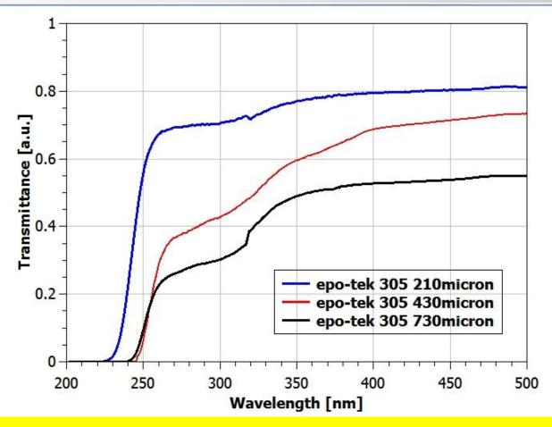
Transmittance curves normalized by the single- quartz support spectrum
