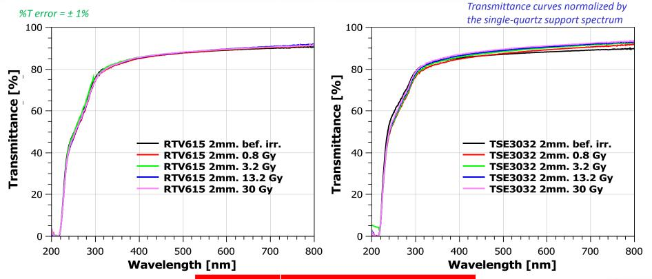
RTV615 and TSE3032: not modified by gamma irradiation (up to 30 Gy)
