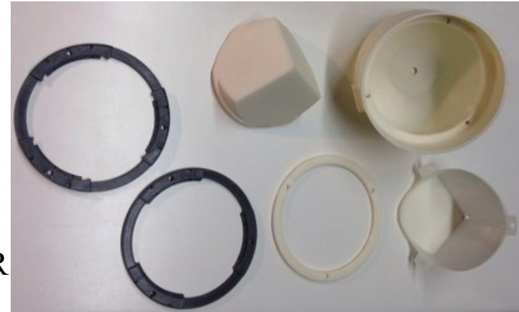
Photos of 3D-printed plastic components of MoonLIGHT
