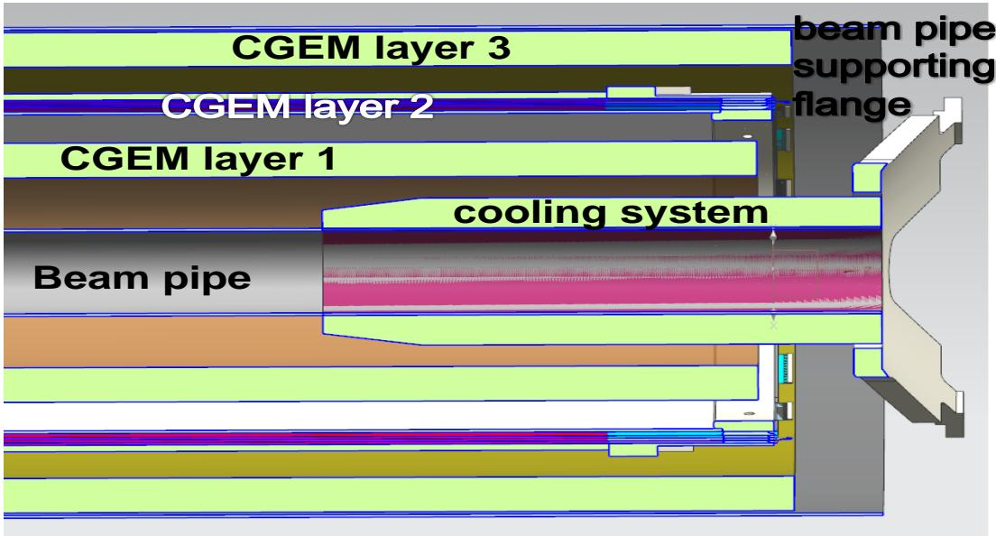
Length of the three layers will be slightly incremental with the radius (Inner radius 78 mm and outer radius 179 mm).
