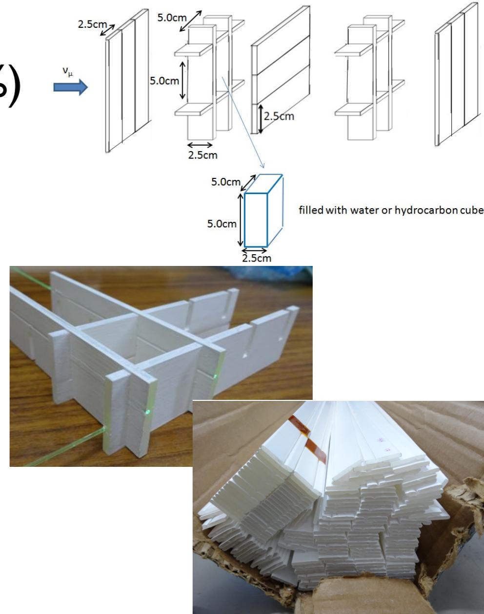
3mm-thick scintillator produced at Fermilab
