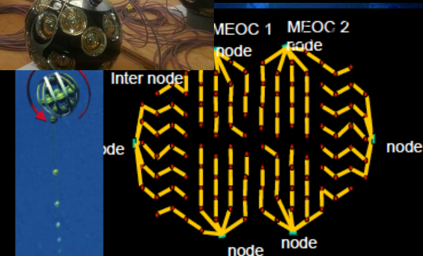
Current optimisation: 0.6 KM3 Blocks of 115 strings, 90m apart, 18 DOM/String, spacing between DOM's 36 m
