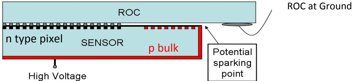
Air gap between sensor and ROC can be as low as  $10\mu\text{m}$  with Indium Bump Bonding: high spark probability
