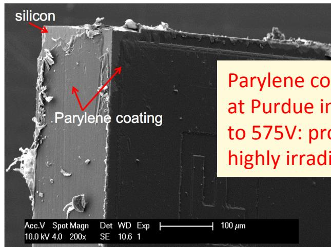
Parylene coating  $2\mu\text{m}$  thick tested at Purdue improves Breakdown up to  $575\text{V}$ : probably not enough for highly irradiated pixel
