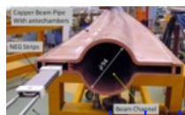
Replace beam pipes with TiN-coated beam pipes with antechambers
