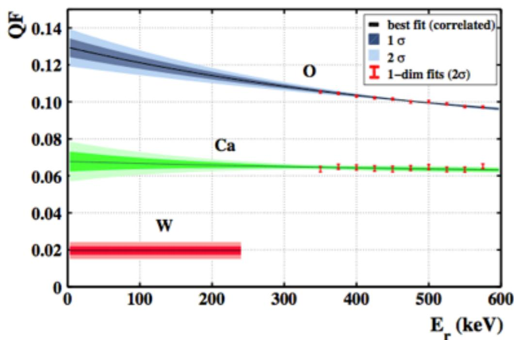
Precise measurement of QF of O, Ca and W at mK temperatures
