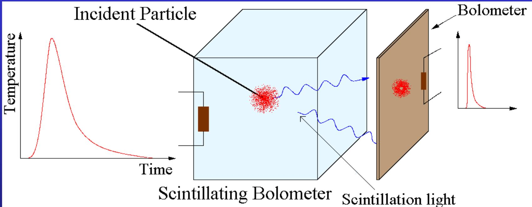
*A Bolometric Light Detector (BLD) is fully active a particle detector*
