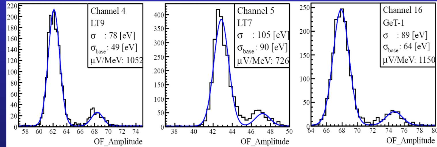
The  $^{55}\text{Fe}$  energy spectra evaluated on three different UMICORE Ge-crystals.  $\sigma$  represents the evaluated energy resolution on the peaks, while  $\sigma_{\text{base}}$  represents the baseline resolution.
