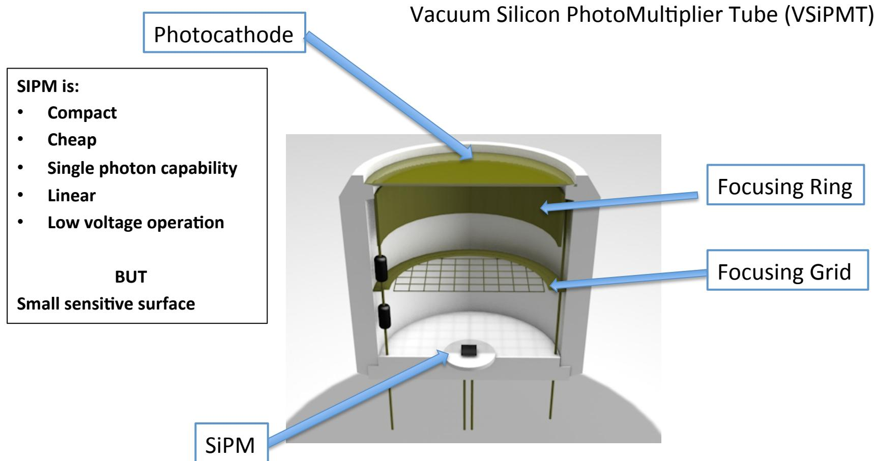
A combination of a classical vacuum glass PMT standard envelope hosting a photocathode and a Silicon PhotoMultiplier (SiPM) acting as an electron multiplying detector
