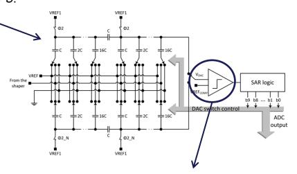
The discriminator is a three stage circuit including a preamplification block and a dynamic latched comparator consisting of a second gain stage and a latch.
