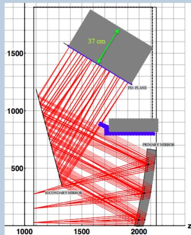
RICH-1 upgrade optical layout optimised using a ray tracing software
