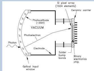
A schematic picture of the Pixel HPD
