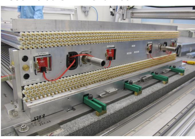
sMDT chambers: newly developed drift tube detectors with 15 mm tube diameter
