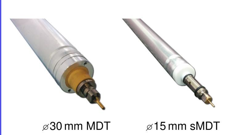
**MDT chambers:** drift tube detectors with 30 mm tube diameter accounting for the majority of precision tracking chambers in the ATLAS Muon Spectrometer
