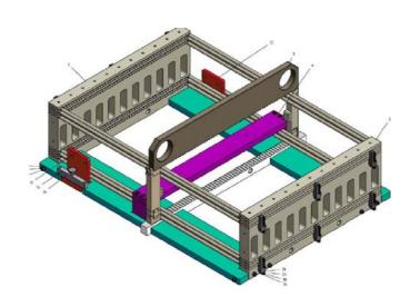
Tube positioning using precisely machined jigs
