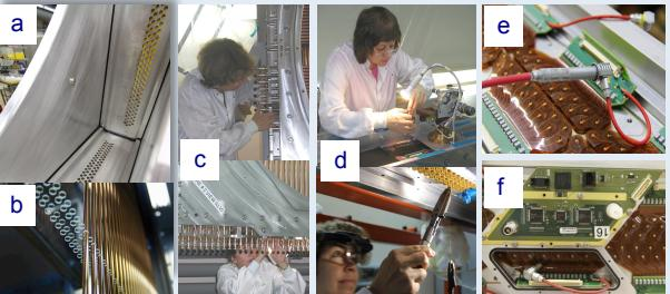
(a) - module sealing by epoxy sealant;
