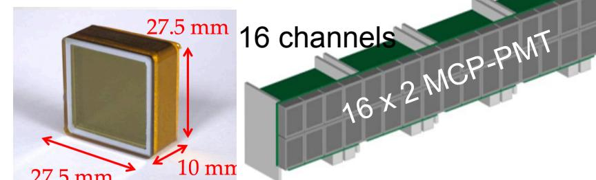
3) front-end readout electronics
