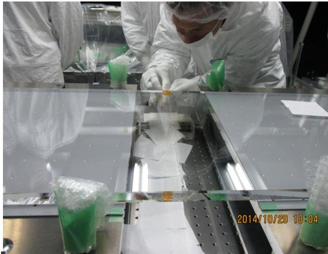
TOP module #1 quartz gluing
