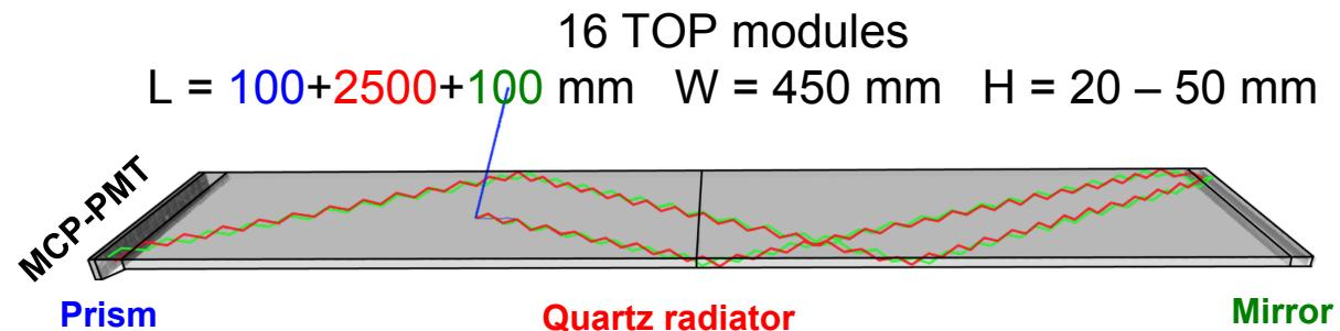
2) micro channel plate (MCP) PMT
