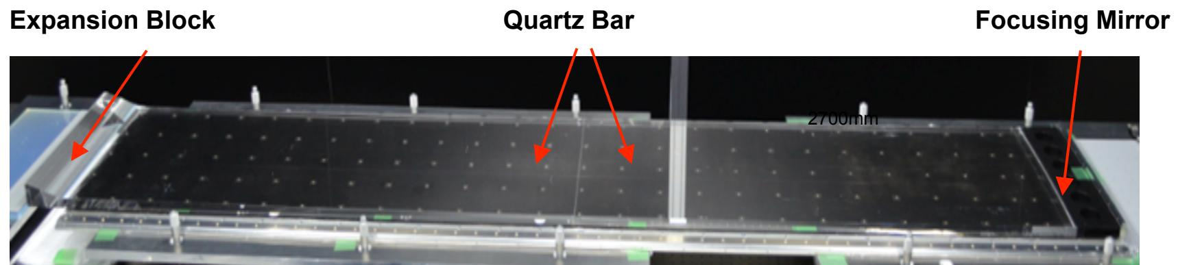
High quality quartz surfaces required for multiple internal photon reflections
