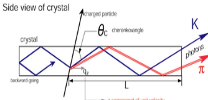
A 2-dimensional PDF can be constructed based on detection time and detection position of Cherenkov photons.
