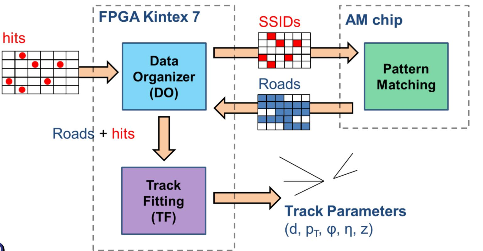
**Track Fitting (FPGA logic)** A fit is done computing all combinations of hits across layers.
